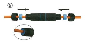
Lock the two waterproof plugs on the cable, then put them into the end of the long tube. Note: The plug is engraved with the word "waterproof" on one side outward.
